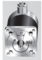
Load angle: Excursion \vartheta of the rotor in reference to the zero position determined by the stator field, in case of a torque M_d at the motor shaft
